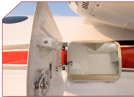
Tail cone Baggage Compartment Height: 457 mm | Width: 603 mm
