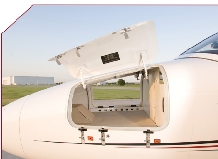
Nose Baggage Compartment: Height: 424 mm | Width: 868 mm
